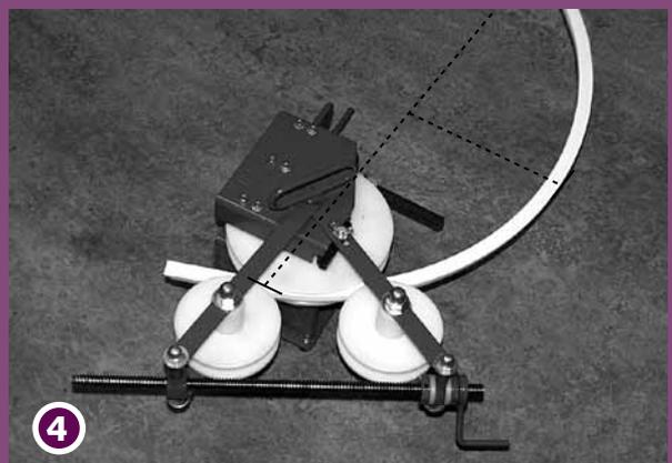
Run the whole distance to be bent through the Continuous Curver until the reference points hit the first Small Bending Dye (A), each time. The radius needs to be checked frequently. If the radius is still not achieved, turn the Small Handle a few times more. Repeat this, until the required radius is created. It is possible to reverse the curve, once the radius is overbent.
