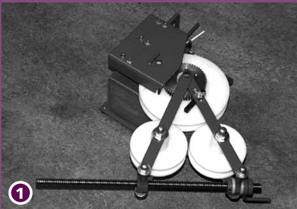
Remove the Metal Pin (C) and the regular bending dye from the Compact Bending tool. Insert the Continuous Curver with the unit Stabilizer (D), so that slack between the Small Bending Dyes (A) and the Compact Bending tool will be avoided.
