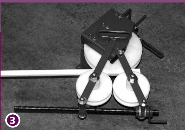
Mark the distance to be bent with reference points on the track. Turn the Small Handle (E) a maximum time of five turns. Start turning the big handle of the Compact Bending tool to bend the track through the Continuous Curver.
