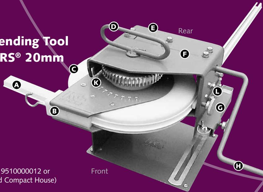
Forest developed one Bending House for: KS, CKS, CRS 20 mm and DS. Depending on the type of track that has to be curved a All-in Bending Wheel can be ordered. Remark: for bending of the CKS track you will need to order the CKS Bending Strip, KS Bending Wheel all-in and a Bending House.
