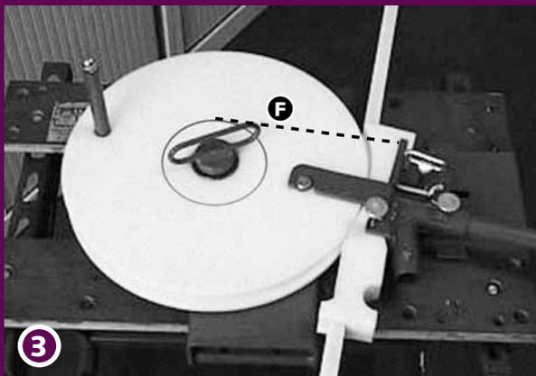
3 Place the Guide-Wedge (C) as depicted on the foto. Slide the track in position and determine the required size from the measurement line (F) to the end of the track. This will create the distance from the outside of the track to the wall.
