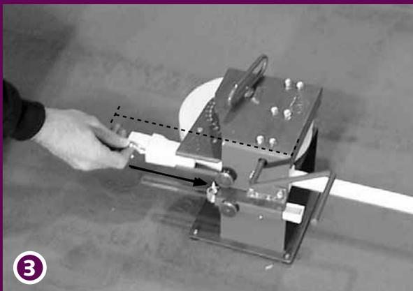
Insert the Guide-Wedge (B) firmly into the place between the metal part of the Bending Dye (C) and the track to position the track in the right place. Take the measurement of the first curve from the end of the Metal House (E) to the end of the track. This will create the distance from the outside of the track to the wall. Start curving by turning the handle (H) clockwise.
