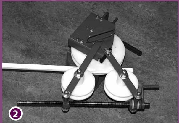
For determining necessary track length  $3,14 \times$  diameter of the circle. Add 10 cm (4") more on both ends. Insert the bending strip into the track. Place the track between the Bending Dyes (A and B) with its slot facing up to make a right hand curve, or down to make a left hand curve. Turn the small handle (E) a few times to avoid slack.
