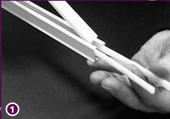
1 First, insert the two smaller bending strips into the track. Then, press the bigger bending strip into the slot of the track between the smaller ones.
