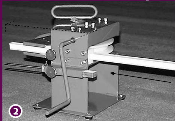
Insert the KS-track through the backside of the Compact Bending tool. To make a right hand curve, insert the track with the slot side up. To make a left hand or reversed curve, insert the track with the slot side down.
