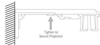
Once desired projection is set for all the brackets, lock the bracket into position by tightening the track depth adjustment set screw (see drawing below).
