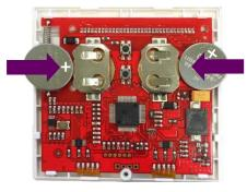
put in the two batteries mind the right polarity
