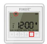
press stop button to enter timing point setting
