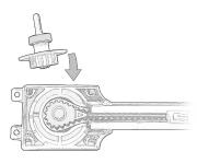
5. Attach Fastener Slide the fastener into the track.
