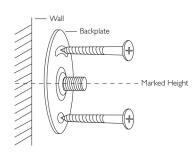
Drill in screws through each hole for a secure mount. Repeat this process for all other brackets evenly spacing them between the two installed brackets.
