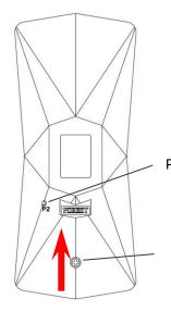
P2 button (for programming tubular motor)
