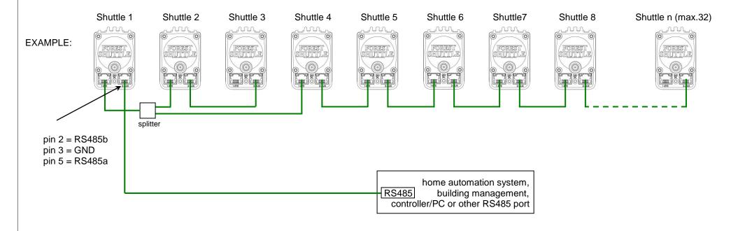
All Shuttles have standard the address 'OWN'. This address can be changed to a unique address before connecting to the FX-bus. Commands are addressed directly to a Shuttle or, in some cases, globally to the entire bus. In order to get a response message from a Shuttle (position ect.) you need to send a request to a unique address. The addressed motor will then respond with a message onto the bus to the Home Automation system / Controller / PC.
