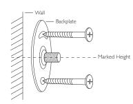
Drill in screws through each hole for a secure mount. Repeat this process for all other brackets evenly spacing them between the two installed brackets.
